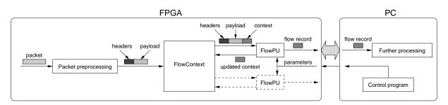
Figure 1: Architecture of the probe
